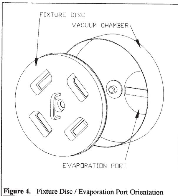
**Figure 4.** Fixture Disc / Evaporation Port Orientation
