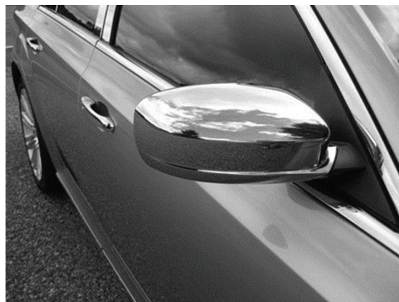
Figure 1. Examples of plating-on-plastic (POP) metallic finishes on the side of an automobile.
