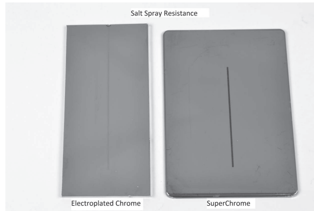
Figure 9: Salt spray resistance test on plaques.
