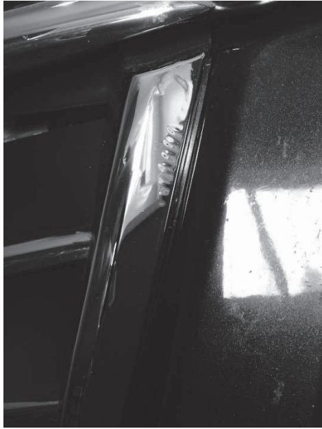
Figure 2: Electroplated chromium delamination.
