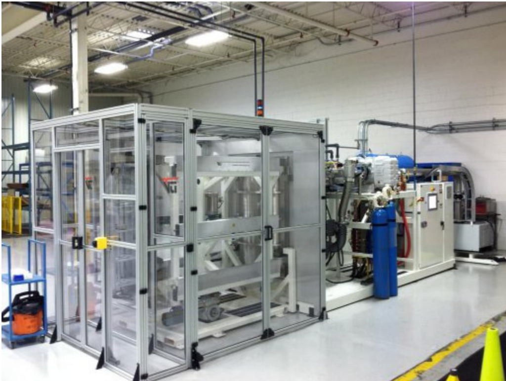
Fig. 3 - Single Point Load VTI Press Side 4000 for high volume sputtered coatings. Photo: Vergason Technology
