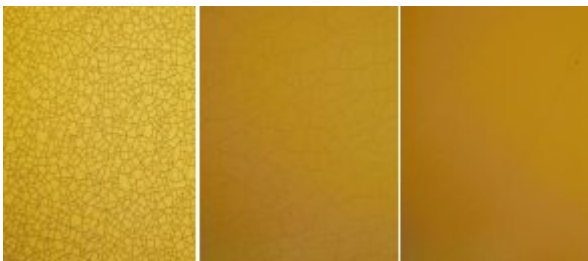
A B C Fig. 4 – Base-coated ABS plaques with 300nm of chrome sputter deposited. Magnification 100X. Chamber pressure maintained at 2 milli-torr during deposition. A: deposition at 310
