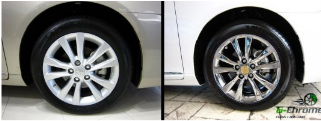
Fig. 7 - Before and after pictures of PVD Chrome on automotive wheels. Photo: Winona PVD Coatings www.g-chrome.com
