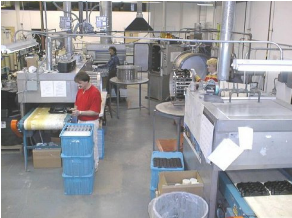
Fig. 2 – Ten parts per minute being cell processed in 1991. Steps included substrate pre-heating to 150°F (near to post molded temperatures), PVD coating of aluminum, paint top coating, and partial thermal cure of painted parts were then sealed in clean containers for full cure during shipment. Mask washer, positioned close the painting machine, could be used without any loss of production time. Photo: Vergason Technology
