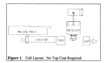
If the metalizer is working as part of a cell, maximum uptime is of the essence. Modular system design allows for quick disconnecting of pumping modules. Systems must be designed so that preventative maintenance tasks such as pump set removal and chamber liner change out can be performed quickly and easily. In larger shops where multiple maintenance entities are required to perform tasks, components must disconnect quickly in order to reduce maintenance time requirements.
